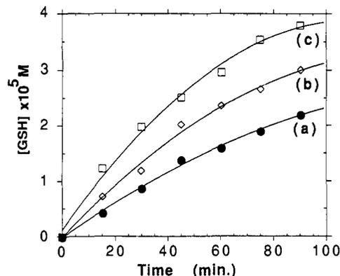
**Figure 1.** Rate of reduced glutathione, GSH, formation using the monolayer enzyme electrodes with different bipyridinium relays. The different curves correspond to bipyridinium units anchored by various spacers to the enzyme: (a) 1a; (b) 1b; (c) 1c. All experiments were performed in a phosphate buffer, pH 7.2, and the applied potential on the working modified electrode was  $E^0 = -0.72$  vs SCE;  $[GSSG] = 1 \times 10^{-2}$  M.
